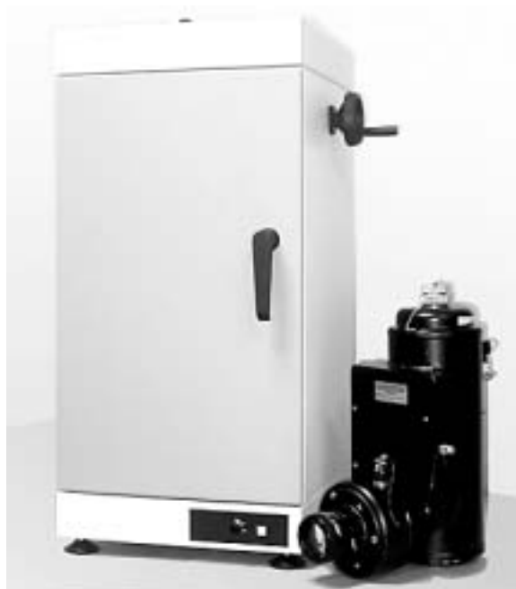
FIGURE 36.2 Dark box imaging system. An example of a dark box setup along with the LN-cooled VersArray 1300B camera that is used to collect chemiluminescence images. During operation, the camera is mounted on the top of the box via a light-tight seal. The box allows macroimaging of chemiluminescence via a movable stage that can be focused from the outside.
