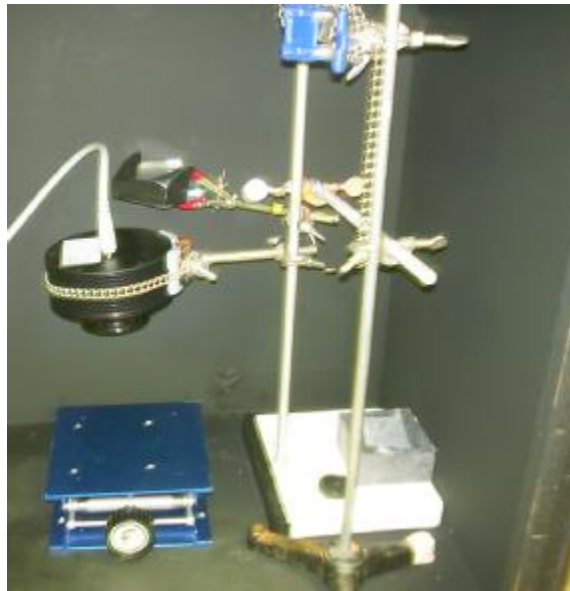
Figure 3: A light tight box (background) contains the imaging apparatus. The ST-6 CCD camera (black) is supported by an adjustable lab stand. A blue lab jack positioned beneath the camera serves as an image bed, and can be vertically adjusted to alter the focal length.
