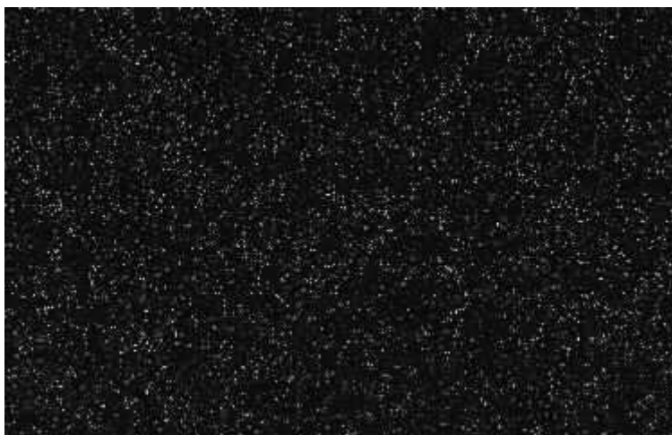
Figure 6: Dark Frame corresponding to Figure 5. This image was taken under the same conditions as figure 5, but with the shutter closed. Note the similarity in figures 5-7.
